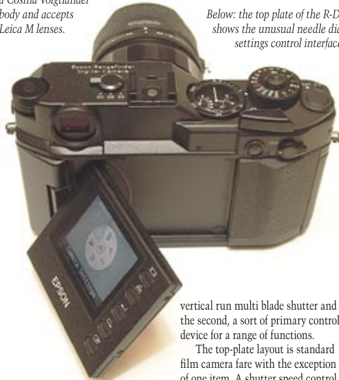
The LCD viewing screen can flip round and seats home like a Leica film camera back panel.
